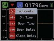
Displays and measures RPM, on time, open time, open delay and close delay.
