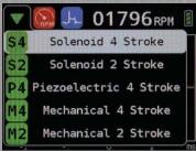
Works on solenoid, piezoelectric and mechanical fuel injectors.
