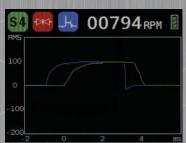
Displays signal voltage, injector power and pintle valve position.
