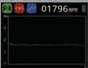
Chart mode used for detecting intermittent or infrequent failures and misfires.
