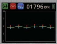
Candle stick graph compares maximum, minimum and average measurements of several injectors.
